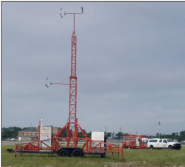
Fig. 1. Florida Coastal Monitoring Program tower platform shown in the foreground. Stowed tower shown in the background.
